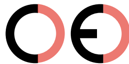
False CE Mark (too far)
